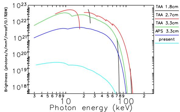
Figure 6: Brightness curves for various 48-m-long undulators in the TAA and an 8-m-long device in the APS, along with the present typical APS performance.
