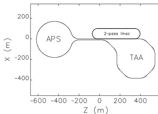
Figure 3: Geometry for the upgrade with very long straights in the TAA.
