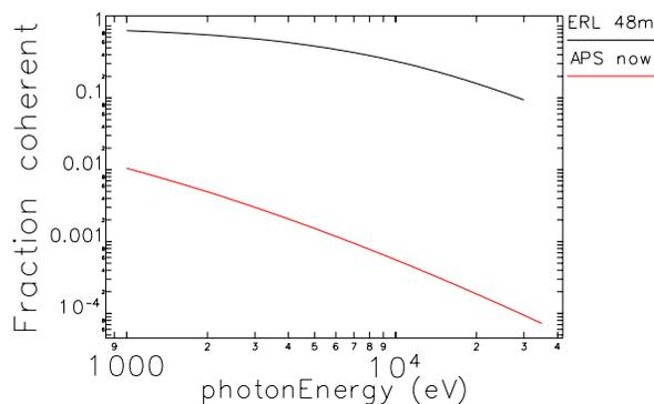
Figure 7: Fraction of radiation that is coherent, for APS today and 48-m-long undulators in the ERL.
