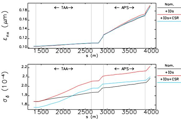
Figure 4: Evolution of horizontal normalized emittance and energy spread in the 7-GeV portion of the system.
