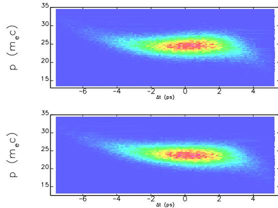
Figure 5: Tracking results at 20 pC/bunch, comparing final longitudinal phase space with (bottom) and without (top) unshielded CSR in dipoles and drifts.
