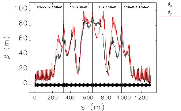
Figure 1: Optics for the two-pass linac, showing acceleration and deceleration stages.
