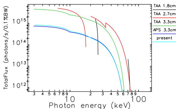
Figure 8: Flux tuning curves for various 48-m-long undulators in the TAA and an 8-m-long device in the APS, along with the present typical APS performance.
