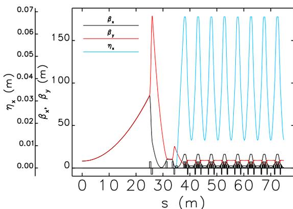
Figure 2: Optics for one half of a TAA octant.
