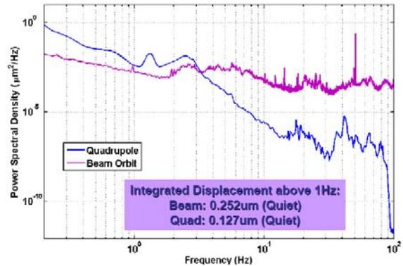
Figure 3: A vertical quadrupole and beam orbit vibration power spectral density comparison at quiet hours.
