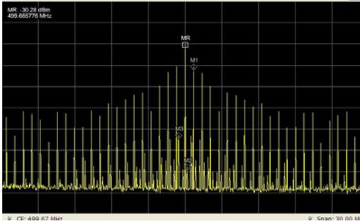
Figure 5: Beam spectrum of the multibunch fill at 64mA.
