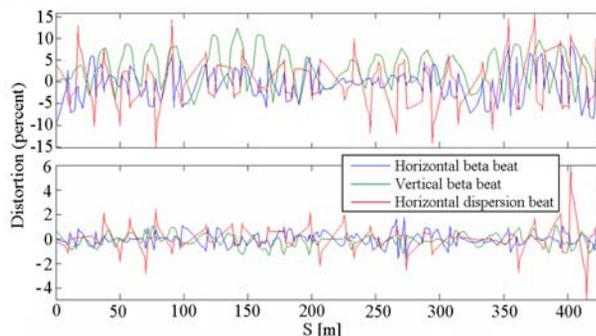
Figure 1: Beta and dispersion beating before (the top plot) and after (the bottom plot) LOCO calibration.
