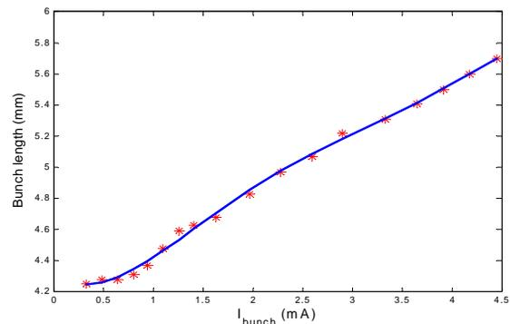
Figure 4: Bunch lengthen with bunch current.
