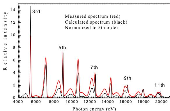
Figure 9: Harmonics of in-vacuum undulator radiation.
