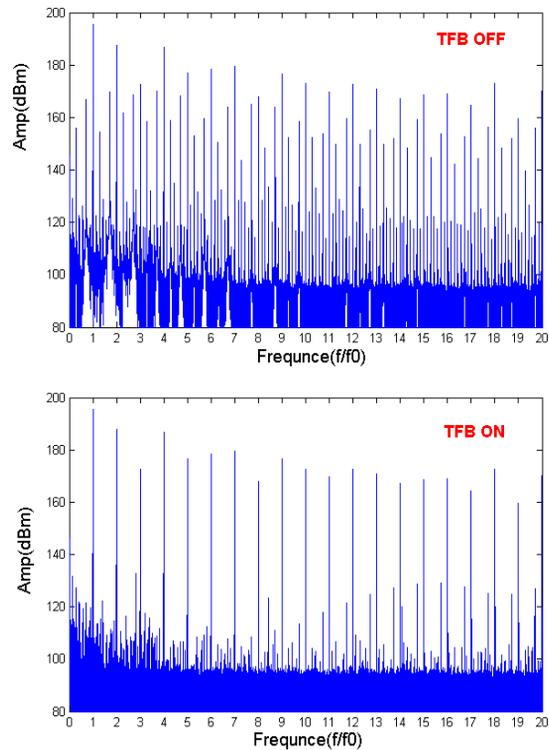
Figure 7: Transverse beam spectrum with TFB off and on (at a beam current of 190mA).
