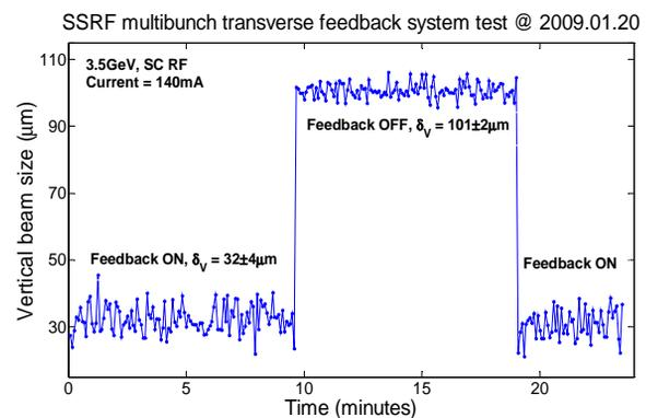
Figure 8: Vertical beam size with TFB on and off.
