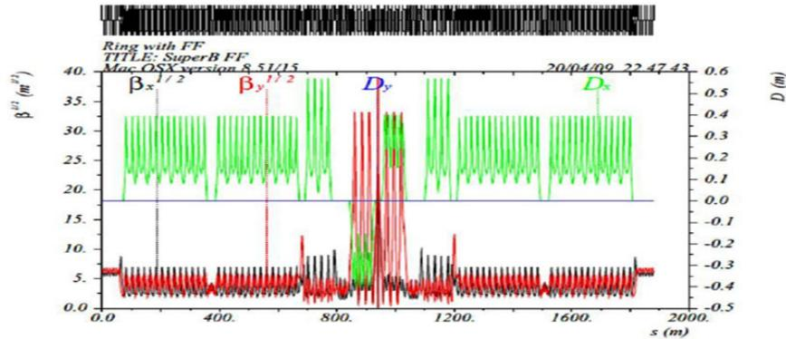
Figure 3: HER optical functions with spin rotator insertions.
