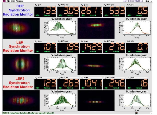
Figure 4: Beam size measurement using an interferometer of synchrotron light in KEKB.
