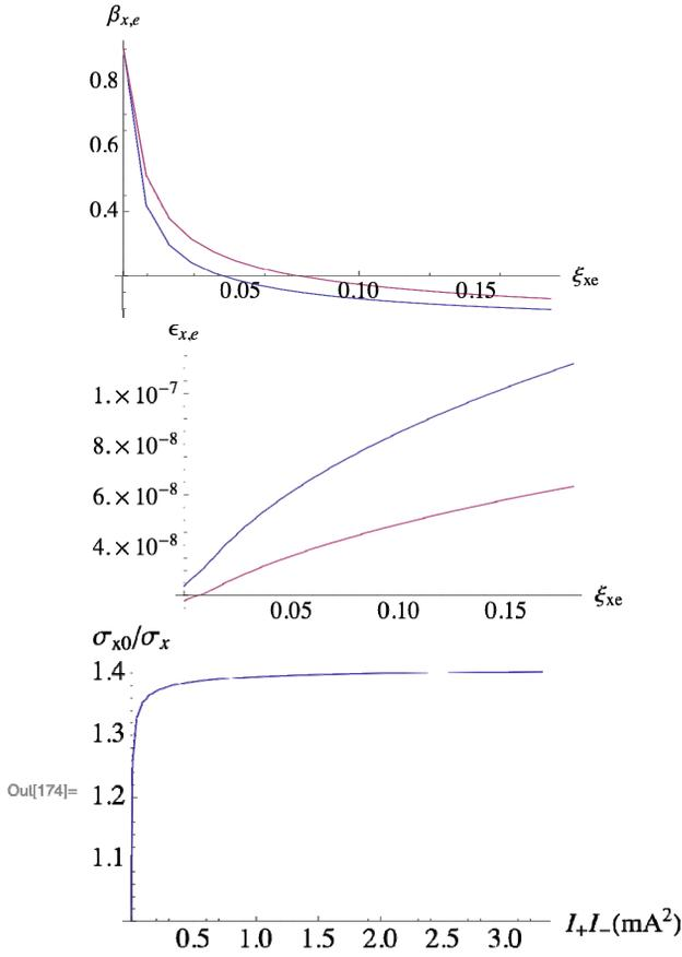
Figure 1: beta function, emittance and beam size ratio for nominal value as functions of nominal beam-beam parameter. The diffusion assignment is  $r=1$ . In the last picture, the horizontal axis is the single bunch current product of the two beams.
