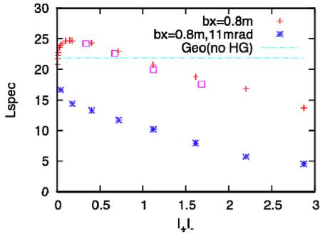
Figure 2: Specific luminosity ( $L/I_+I_-/N_{\text{bunch}}/1026$ ) in KEKB given by a strong-strong simulation. The horizontal axis is the single bunch current product of the two beams.
