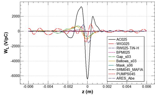
Figure 3: The calculated longitudinal wake functions for various impedances of SuperKEKB LER for  $R = 25$  mm beam pipes with antechambers. The highest peak is still given by the CSR in the arc (black). Then the resistive wall with TiN coating (purple) becomes comparable to the CSR in the wigglers (red-dashed). Bellows (gold), and gaps between beam pipes (green) follow.
