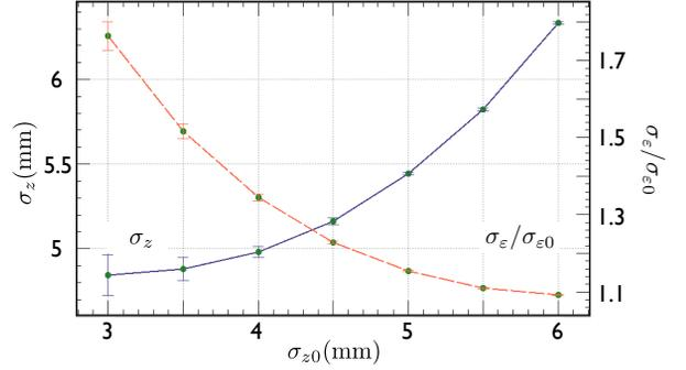
Figure 8: The bunch length (blue, left axis) and the relative momentum spread (red, right axis) at the design intensity as functions of the bunch length at zero intensity. A negative momentum compaction factor is assumed to set  $\nu_s = +0.022$ . The radius of the beam pipe is  $R = 45$  mm.
