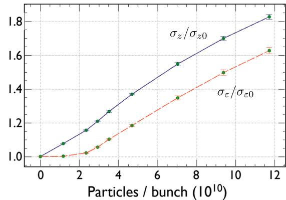
Figure 4: The results of particle tracking simulation with all calculated wakes with the  $R = 45$  mm beam pipe with antechambers, showing the bunch length  $\sigma_z$  and the energy spread  $\sigma_\epsilon$  relative to their zero-intensity values  $\sigma_{z0}$  and  $\sigma_{\epsilon0}$ , plotted against the number of particles per bunch  $N$ . The right most points correspond to the design intensity of the SuperKEKB LER.
