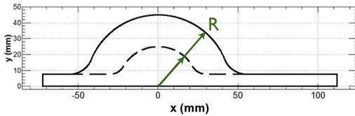
Figure 1: Cross section of the beam pipe with antechambers for SuperKEKB. Two possible shapes with different radii,  $R = 45$  mm (solid) and  $R = 25$  mm (dashed) are shown. The pipe is symmetric to the horizontal plane. The beam is at the origin.
