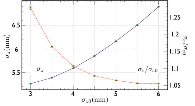
Figure 7: The bunch length (blue, left axis) and the relative momentum spread (red, right axis) at the design intensity as functions of the bunch length at zero intensity. The radius of the beam pipe is  $R = 25$  mm.
