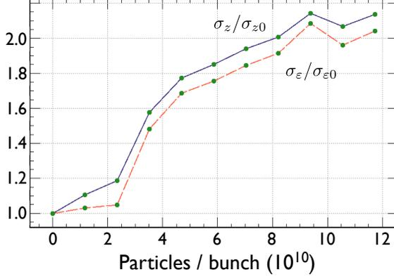
Figure 5: The microwave instability estimated by examining the stability of the Vlasov equation with the same condition as the tracking in Fig. 4, showing the bunch length  $\sigma_z$  and the energy spread  $\sigma_\varepsilon$  relative to their zero-intensity values  $\sigma_{z0}$  and  $\sigma_{\varepsilon0}$ , plotted against the number of particles per bunch  $N$ . The threshold of the instability,  $N \sim 2 \times 10^{10}$  is consistent with tracking.
