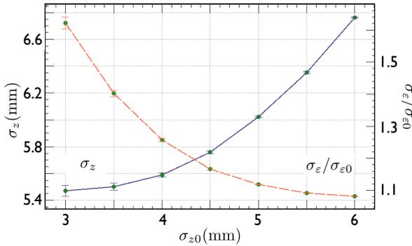
Figure 6: The bunch length (blue, left axis) and the relative momentum spread (red, right axis) at the design intensity as functions of the bunch length at zero intensity. The radius of the beam pipe is  $R = 45$  mm.
