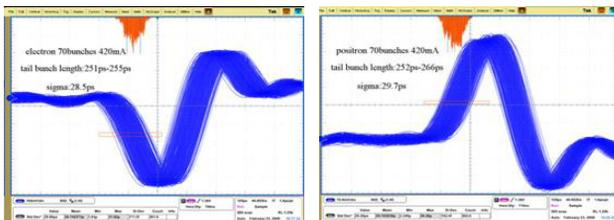
Figure 9: Longitudinal oscillation after the SM's removed. Left:  $e^-$  bunches Right:  $e^+$  bunches
