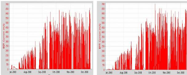
Figure 5: Current growth during the phase 3 commissioning in 2008, BER (left) and BPR (right).
