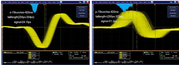
Figure 7: Longitudinal oscillation for bunch train tail. Left:  $e^-$  bunches Right:  $e^+$  bunches
