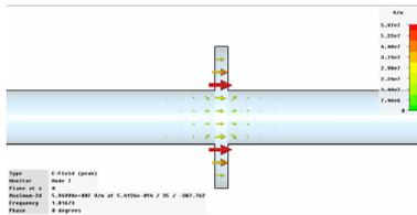
Figure 8: Trapped mode at a flange gap of the SM's.
