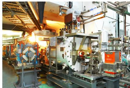
Figure 3: A superconducting RF cavity in installation.
