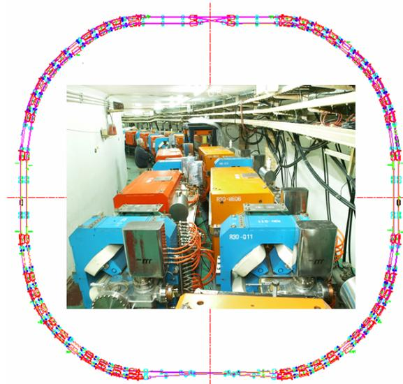
Figure 1: Layout and installed double-ring units.
