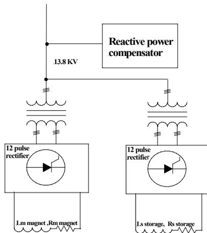
Figure 3: Two thyristor control supplies interfaced with a magnet and a storage inductor.
