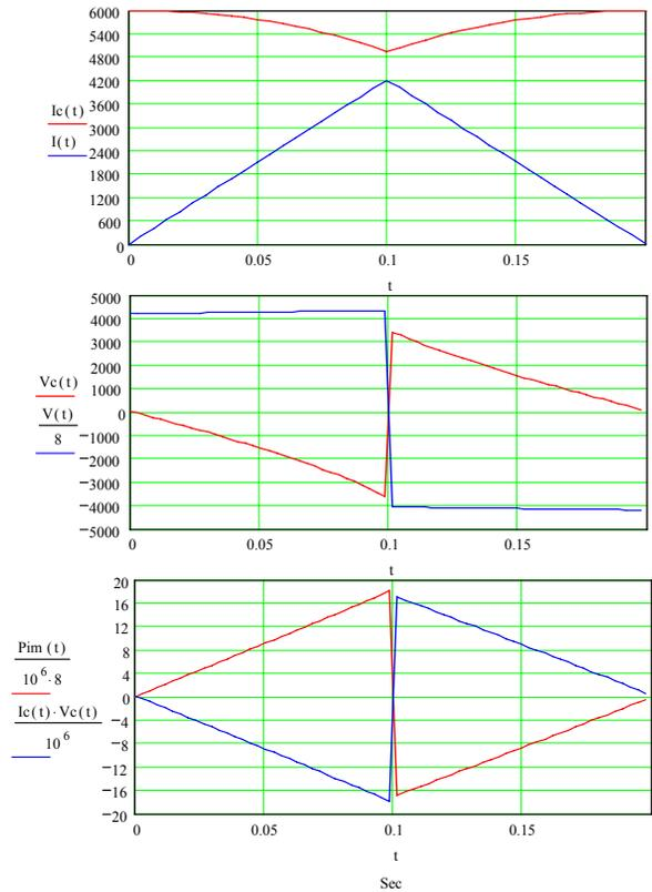
Figure 4: Inductor storage wave forms, for 5 Hz operation.
