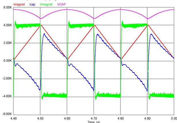
Figure 9: Magnet current and voltage, capacitor current and voltage for 5 Hz operation.
