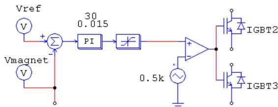
Figure 8: Two quadrant converter control system.
