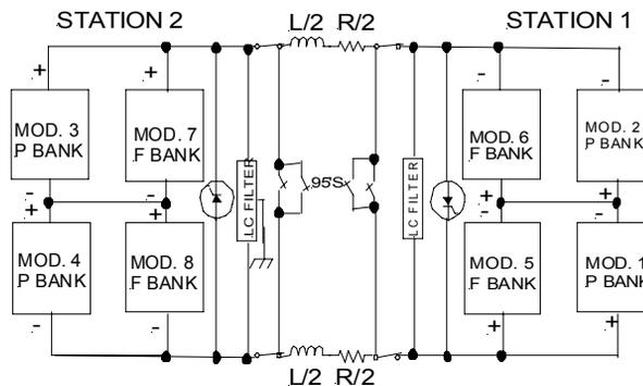
Figure 1: Present AGS Magnet Power Supply.
