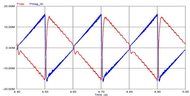
Figure 10: Capacitor and magnet peak power waveforms for 5 Hz operation.
