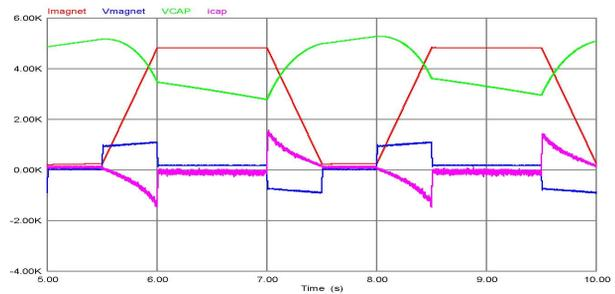
Figure 11: Magnet current and voltage, capacitor current and voltage for present operation.
