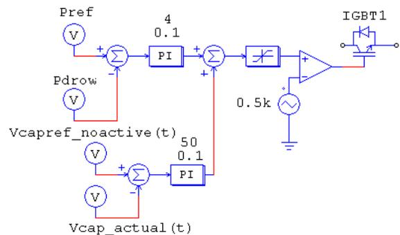
Figure 7: Buck converter control system.
