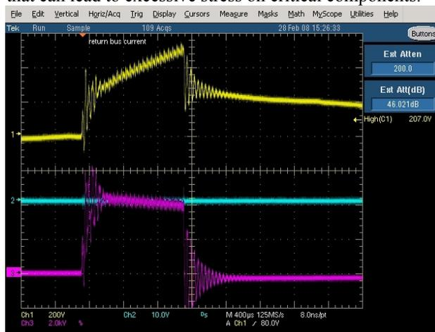
Figure 6: Capacitor Return Current Waveforms. Channel 1 (yellow) is the return bus current at 200 A/div and Channel 3 (magenta) is the energy storage capacitor current at 2000 A/div.
