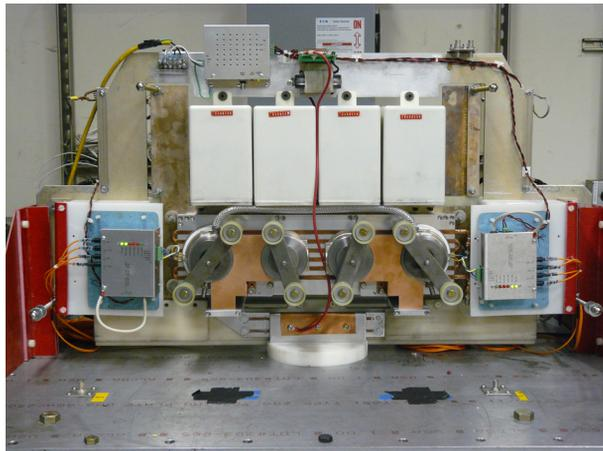
Figure 5: Retrofittable Westcode Press Pack IGBT Assembly with External Antiparallel Diodes.
