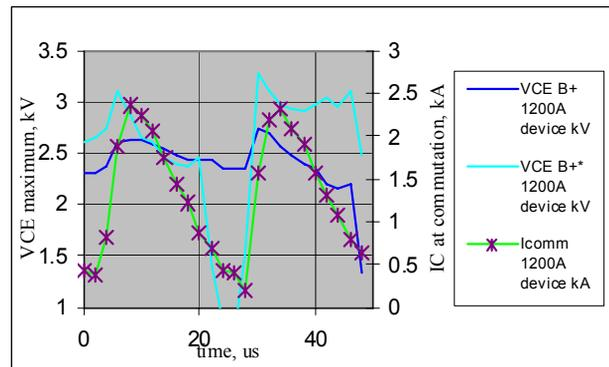
Figure 4: IGBT  $V_{CE}$  Over-Voltage Variations with Commutated Collector Current on the H-Bridge.
