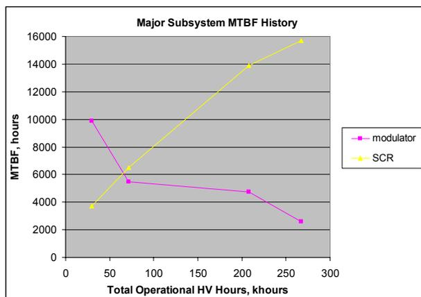
Figure 2: Evolution of Reliability for Modulator Subsystems.
