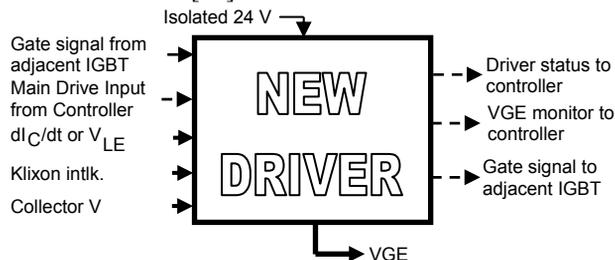
Figure 3: Functional Block Diagram of Next Generation IGBT Gate Drive Circuit.
