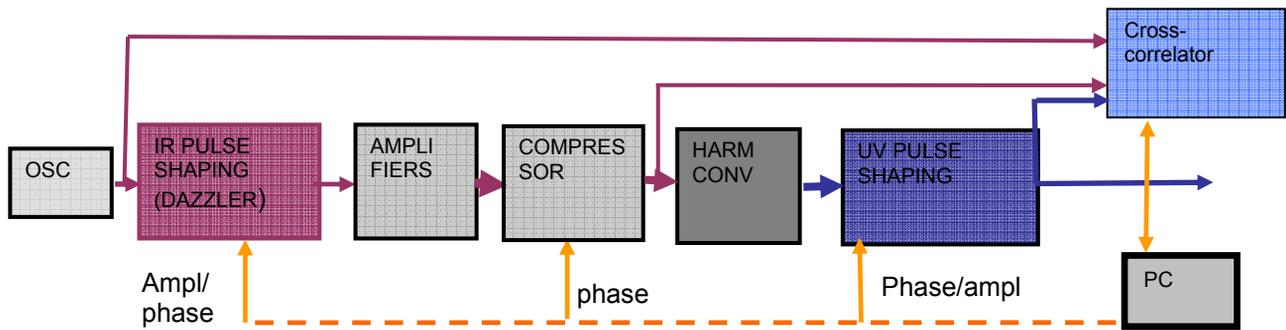
Figure 1: Layout of the pulse shaping system for the FERMI photoinjector laser.
