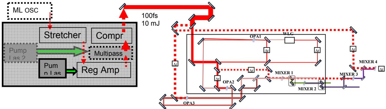
Figure 2: Optical Layout of the FERMI seed laser, upgrades in dashed line.
