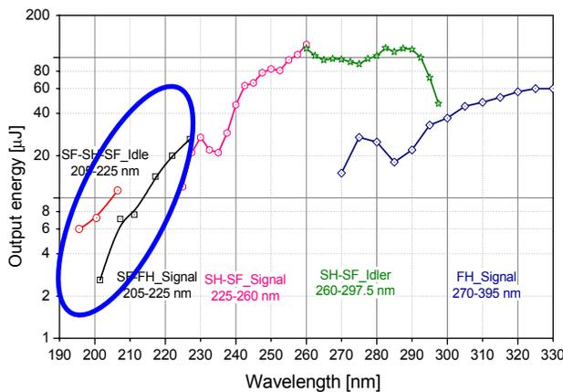
Figure 3: Present tuning curve of the FERMI seed laser.
