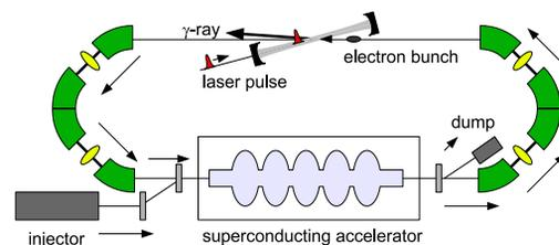
Figure 2: LCS  $\gamma$ -ray source based on an ERL.
