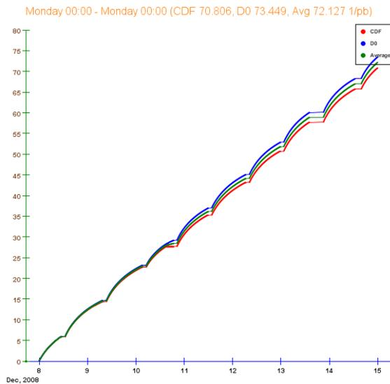
Figure 5. Record integrated luminosity for the week of December 8<sup>th</sup> 2008 was generated using the strategy described for cycling a store.
