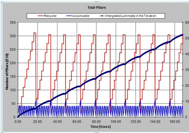
Figure 2: Stacking /Stash sequence over 168 hour period.
