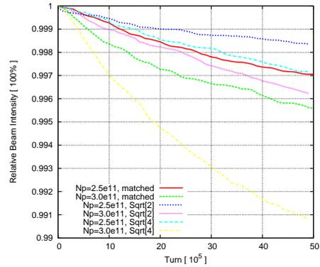
Figure 5: Particle loss with unmatched electron beam size.
