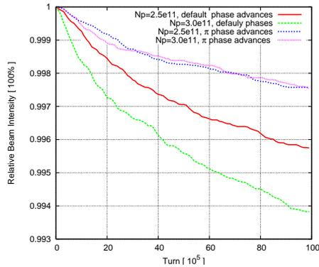
Figure 4: Particle loss with  $N_p = 2.5 \times 10^{11}$  and  $3.0 \times 10^{11}$ .
