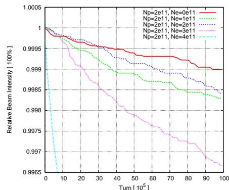
Figure 2: Beam-beam compensation with  $N_p = 2 \times 10^{11}$ .
