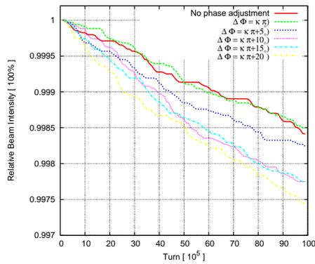
Figure 3: Phase adjustment between IP8 and IP10.
