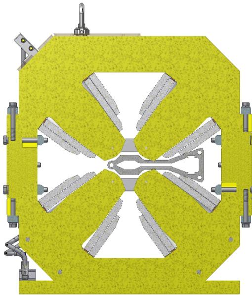
Figure 1: 90 mm Aperture Quadrupole.
