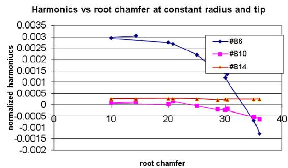
Figure 6: Harmonics versus root chamfer.
