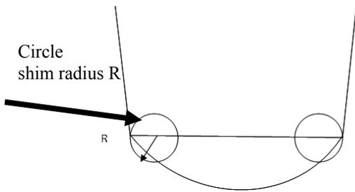
Figure 2: Termination of transverse pole profile with circular shim.
