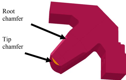
Figure 3: Tip and root chamfers.
