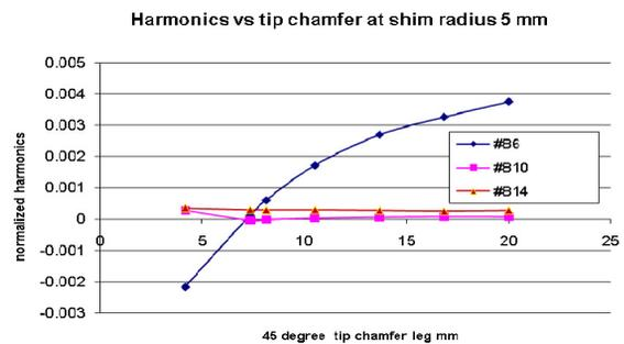
Figure 5: Harmonics versus tip chamfer.
