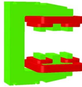
Figure 5: 3D Design- 156mm corrector without the skew quadrupole coils.
