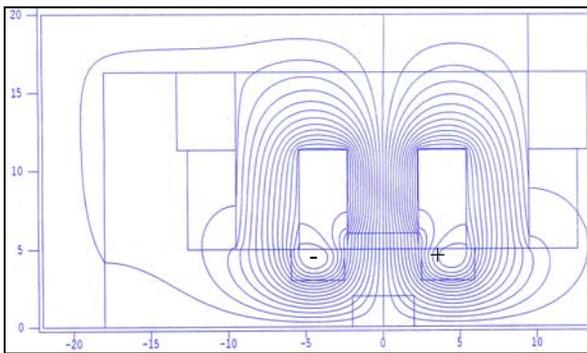
Figure 4: Skew quadrupole corrector.
