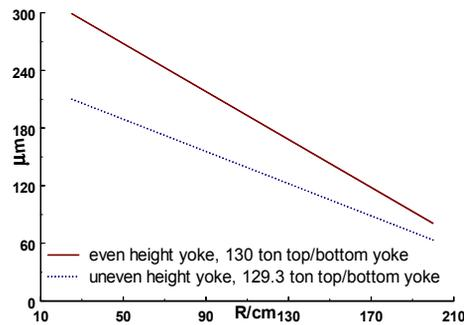
Figure 4: The result of deformation for different structure.
