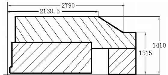
Figure 5: The structure of the uneven height yokes.
