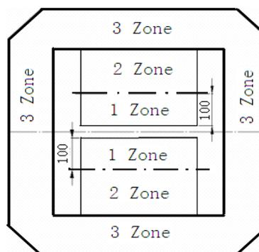
Figure 2: Three zones for ultra-sonic detection.
