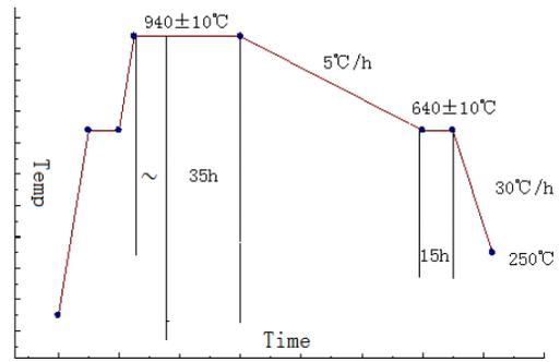
Figure 3: Draft of heat treatment technics.
