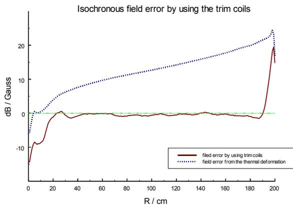
Figure 6: Filed adjust when the temperature changes by 25°C.
