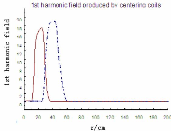
Figure 2: The 1<sup>st</sup> harmonic fields produced by each set of centering coil ( $\pm 100\text{A}$  of opposite coil, rest are 0A)
