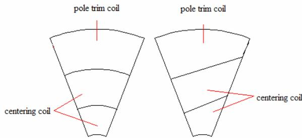
Figure 1: The configuration of the coils on the pole face.
