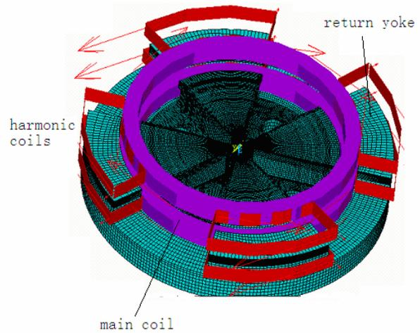
Figure 3: Harmonic coils on the return yoke.
