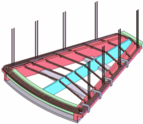
Figure 4: Configuration of the trim coils.
