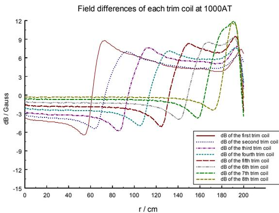
Figure 5: Filed effect of each trim coil at 1000AT.
