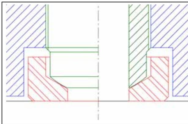
Figure 1: The leg consists of the fine-thread screw and the horseshoe-part.
