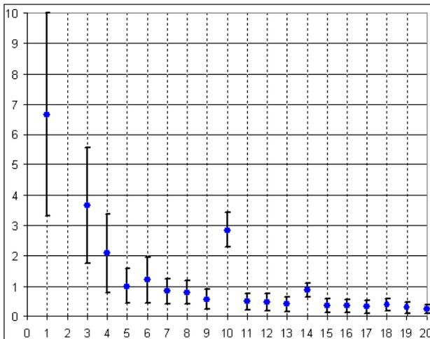
Figure 4: The statistical results of  $\sqrt{A_n^2 + B_n^2} / \sqrt{A_2^2 + B_2^2}$  for the first twenty harmonics on 114 serial quadrupoles at 150A. In units 0.0001.
