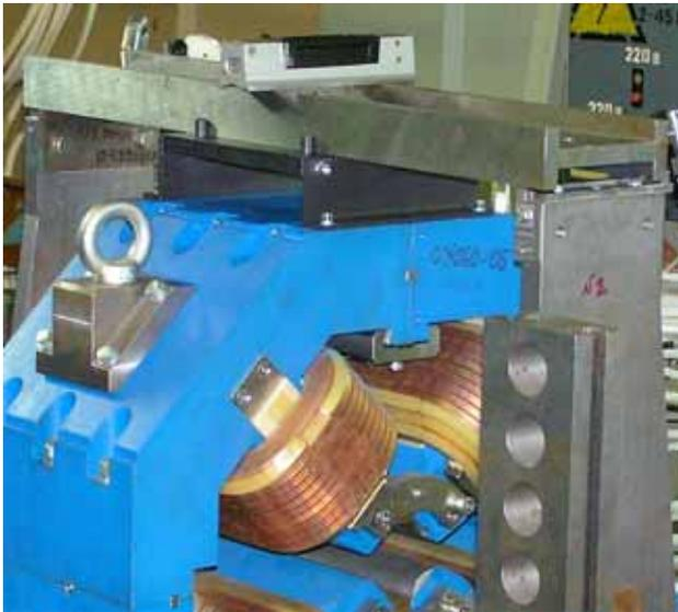
Figure 2: The alignment of the plates for the alignment marks on a quadrupole.
