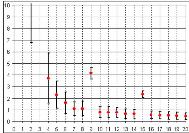
Figure 5: The statistical results of  $\sqrt{A_n^2 + B_n^2} / \sqrt{A_3^2 + B_3^2}$  for the first twenty harmonics on 122 serial sextupoles at 150A. In units 0.0001.
