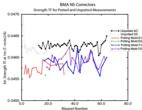
Figure 3: Sextupole strength transfer function versus the BMA production number.
