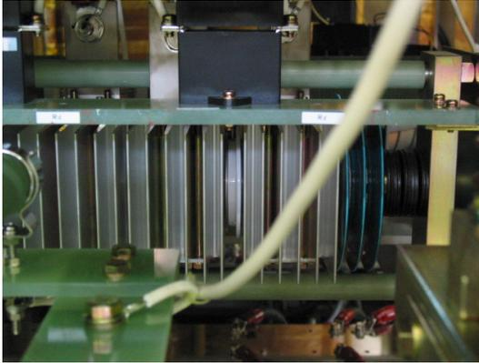
Figure 6: Switching thyristor of the power supply.
