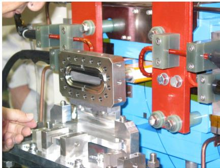
Figure 3: Special removable flange of the ceramic chamber.
