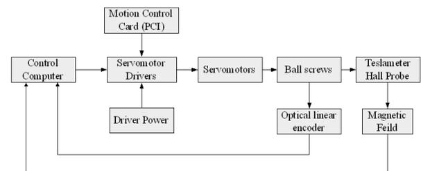
Figure 4: Block diagram of measurement and motion control system.
