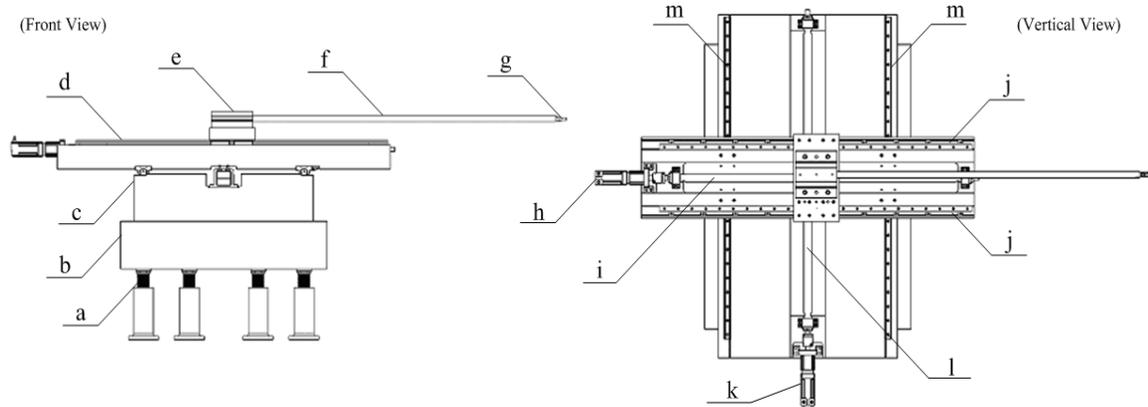
Figure 3: Concise view of the magnetic field measurement system. a: the alignment support; b: the reference plane; c: x-axis plane; d: y-axis plane; e: Hall probe carrier; f: supporting rod; g: Hall probe; h: y-axis motor; i: y-axis ball screw; j: y-axis guide rail; k: x-axis motor; l: x-axis ball screw; m: x-axis guide rail.
