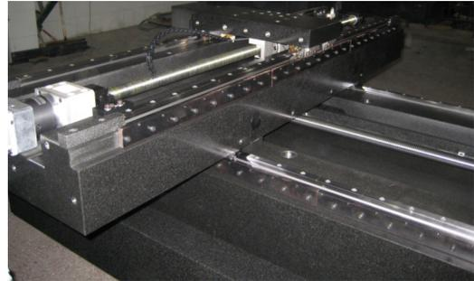
Figure 6: Granite x-y motion stage.
