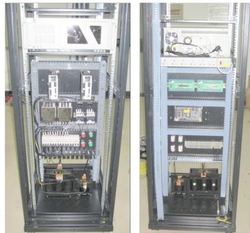
Figure 7: Control cabinet for the measurement system.
