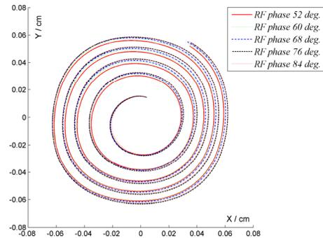
Figure 7: Beam trajectories of first 5 turns with  $32^\circ$  RF phase width
