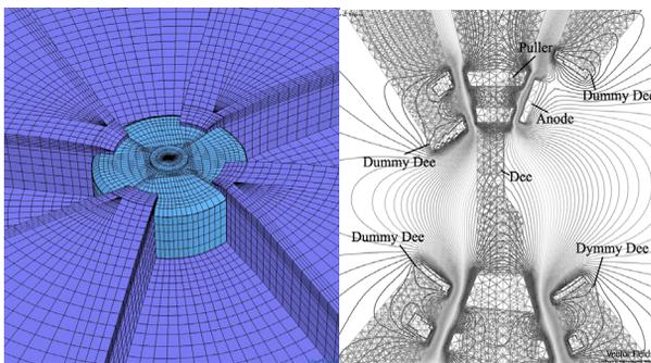
Figure 6. The central magnet and dee structure
