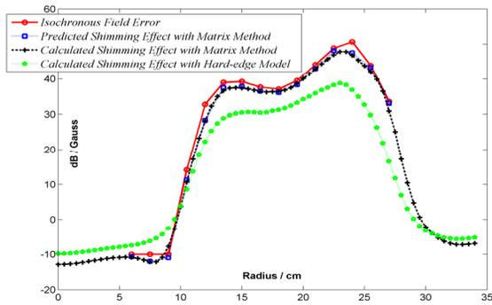
Figure 4: Compare of the shimming effect of two methods
