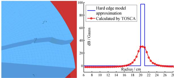
Figure 2: Compare of the hard edge approximation and the realistic field change for a cutting block.
