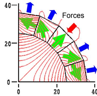
Figure 5: The magnetic forces on magnet segments. Only the segments at pole positions are attracted inside, and the others are repelled towards outside.
