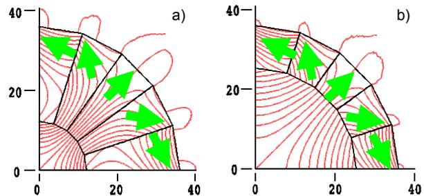
Figure 2: Segment Layouts with the outer diameters of 72 mm. a) for ILC with 22mm bore diam.. b) for ATF2 with 50mm bore diam. The field gradients are 140T/m and 30T/m, respectively.
