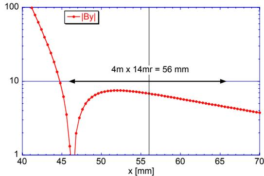
Figure 4: External field for the 20-segmented PMQ.
