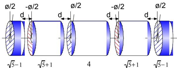
Figure 1: The five-ring-singlet. The odd numbered rings and the even numbered rings are rotated against each other. The values shown at the bottoms of the rings are concluded by R.L. Gluckstern in a case of  $d = 0$  (the rings touch each other).
