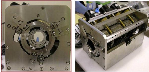
Figure 9: Fabricated five-ring-singlet quadrupole magnet. Left: A hole for the outgoing beam position is located. Right: Three ultrasonic motors drive the rings; even numbered rings are connected together and driven by the center motor.
