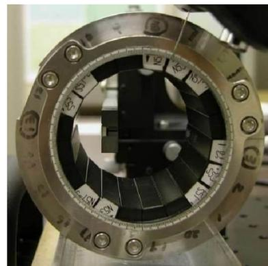
Figure 7: One out of five assembled PMQ's.
