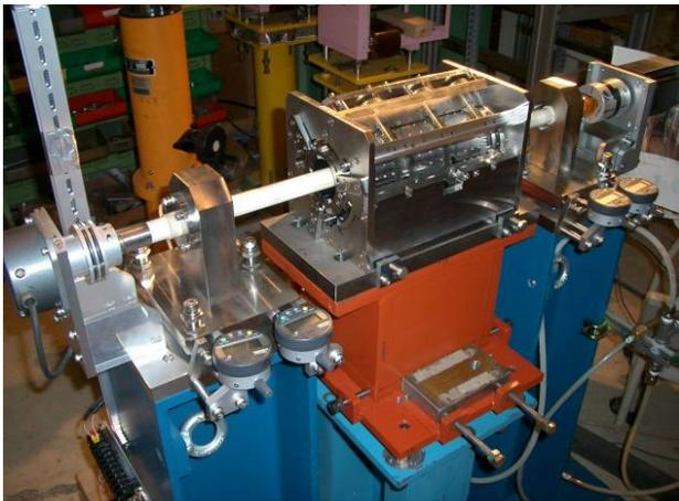
Figure 10: Rotating coils system at KEK.
