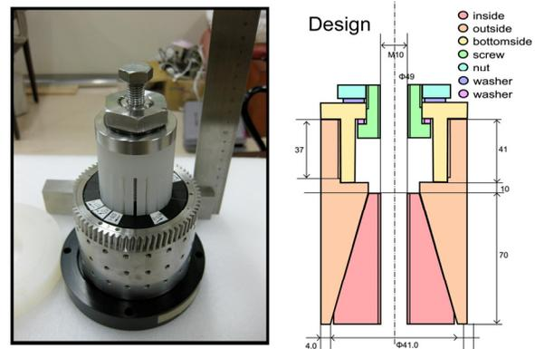
Figure 6: Special jig to fine adjust the position of the magnet segments.
