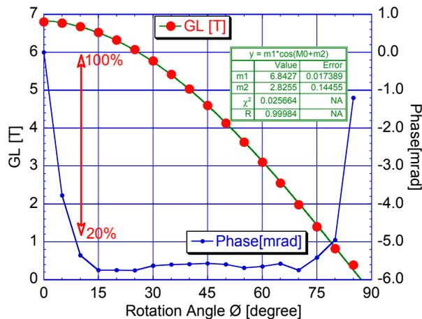
Figure 11: Integrated field gradient as a function of the rotation angle. The quadrupole plane tilt is also plotted.
