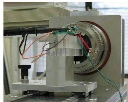
Figure 8: Magnetic center measurement.
