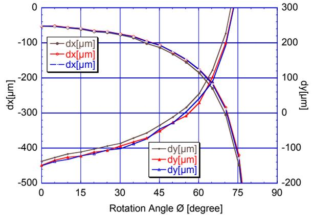
Figure 12: Magnetic center excursion as functions of the rotation angle. Three lines correspond to three runs of measurements.
