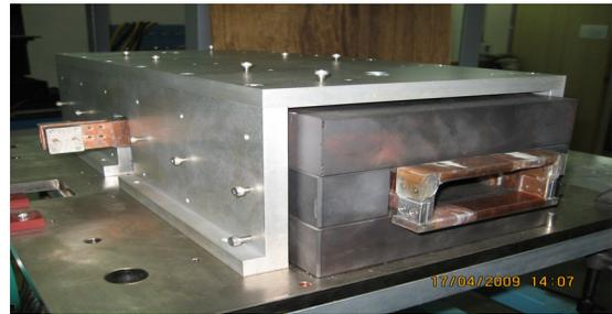
Figure 2: The prototype of the storage ring kicker magnet.
