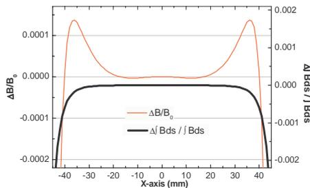
Figure 2: Field homogeneity of central and integral fields of the quadrupole magnet in the transverse direction;  $\Delta B/B_0 = [B(x)-(b_0 + b_1x)]/B(x)$  and  $\Delta \int Bds / \int B_0ds = [\int B(x)ds - (B_0 + B_1x)] / \int B(x)ds$ .
