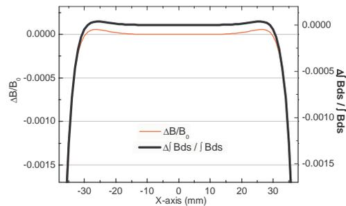
Figure 3: Field homogeneity of central and integral fields of the sextupole magnet in the transverse direction;  $\Delta B/B_0 = [B(x)-(b_0 + b_1x + b_2x^2)]/B(x)$  and  $\Delta \int Bds / \int B_0ds = [\int B(x)ds - (B_0 + B_1x + B_2x^2)] / \int B(x)ds$ .
