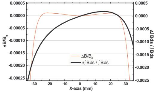
Figure 1: Field homogeneity of central and integral fields on the transverse  $x$ -axis;  $\Delta B/B_0 = [B(x)-B(0)]/B(0)$  and  $\Delta \int Bds / \int Bds = [\int B(x)ds - \int B(0)ds] / \int B(0)ds$ .
