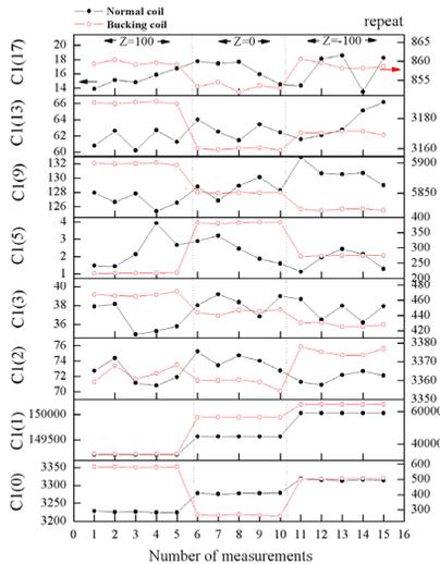
Figure 4: Systematic error test of the normal and bucking coils. The errors for the normal and bucking coils are plotted with lines through the solid (black) and open (red) circles, respectively.
