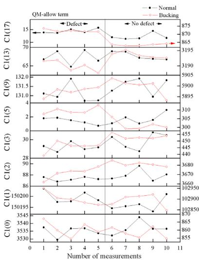
Figure 5: Artificial defect test spectra of the allowed term measured with the normal (black) and bucking (red) coils.
