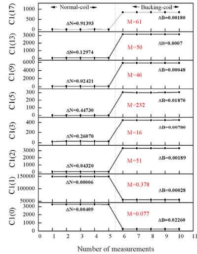
Figure 3: Systematic reproducibility ( $\Delta$ ) and signal magnification ( $M$ ) of the normal and bucking coils when the coil was reinstalled.
