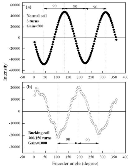
Figure 2: (a) and (b) show measured spectra of the normal and bucking coils.
