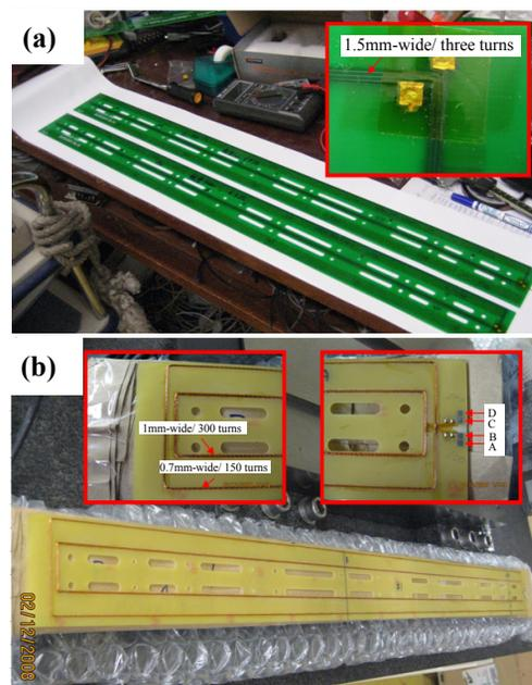
Figure 1: (a) and (b) are photographs of the normal and bucking coils, respectively. The normal coil has three turns and a width 0.3 mm per coil. The bucking coils have 150 and 300 turns with diameter 0.05 mm per coil.
