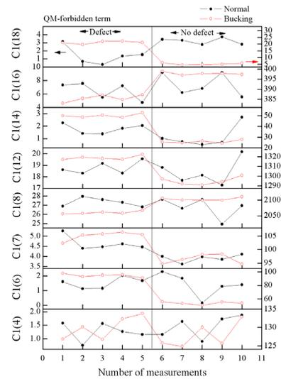
Figure 6: Defect test spectra of the forbidden term measured with the normal (black) and bucking (red) coils.
