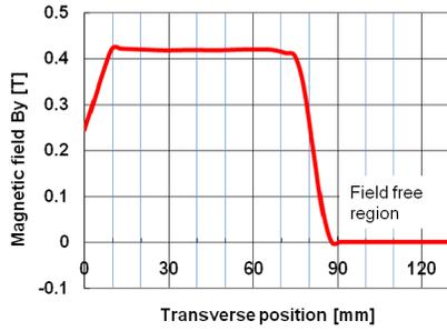
Figure 3: Magnetic field distribution of the injection septum on the midplane.
