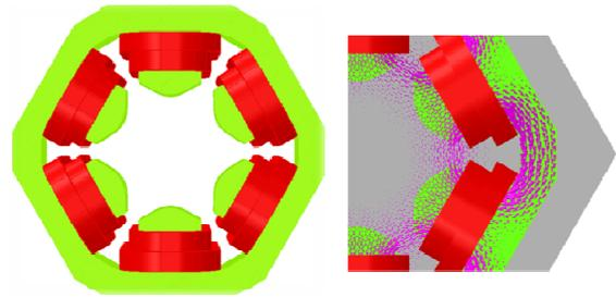
Figure 9: FEM model of sextupole and flux profile.
