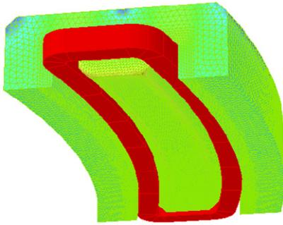
Figure 7: FEM 1/2 Model of Dipole Magnet.
