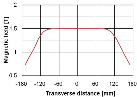
Figure 8: Field uniformity of dipole magnet.
