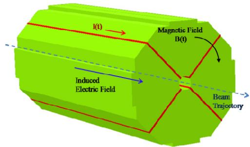
Figure 5: Schematic view of the betatron core.
