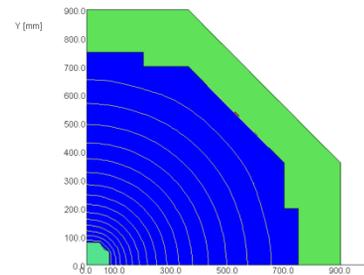
Figure 6: Flux lines inside betatron core.
