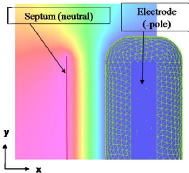
Figure 4: Potential contours of the electrostatic extraction septum.
