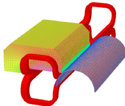
Figure 2: FEM 1/4 model of injection septum.
