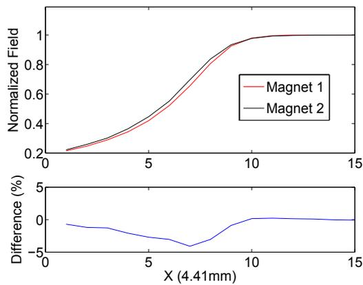
Figure 7: Fringe fields at the entrance of dipoles #1 and #2 and its differences.
