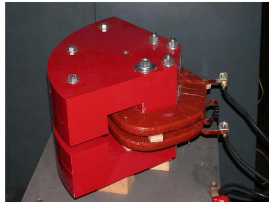
Figure 2: Photo of one of the 90° bending magnets.
