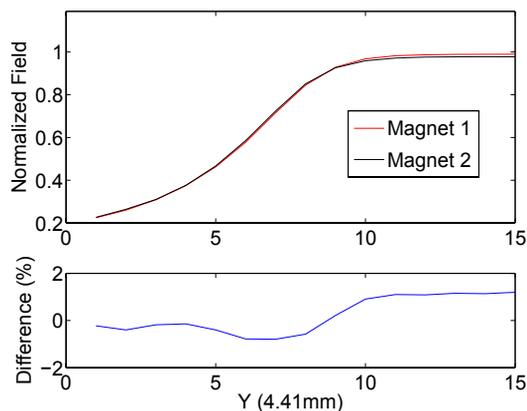
Figure 8: Fringe fields at the exit of dipoles #1 and #2 and its differences.
