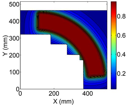
Figure 3: Normalized field distribution of the dipole #1.
