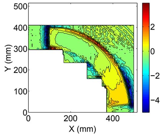
Figure 5: Field distribution differences between dipoles #1 and #2. Color scale in percent.
