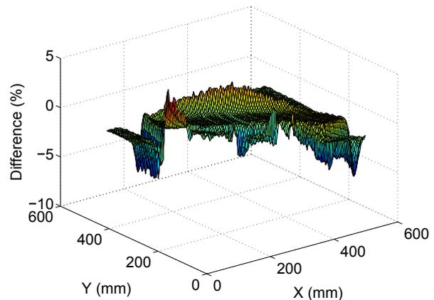
Figure 6: Tri-dimensional graph of field distribution differences between dipoles #1 and #2.
