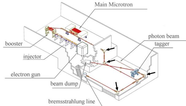
Figure 1: Lay-out of the accelerator and the positions of the 90 bending magnets.
