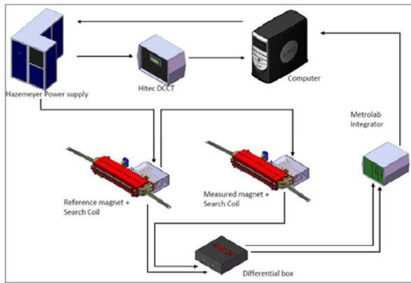
Figure 3: Measurement chain.
