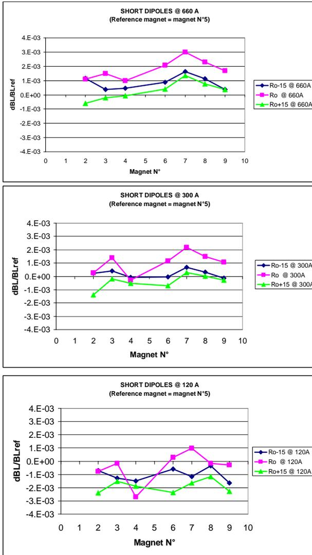
Figure 7: Short dipoles measurement @ 120, 300 and 660 A.
