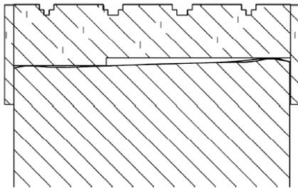
Figure 4: Search coil support (upper yoke not shown for clarity).
