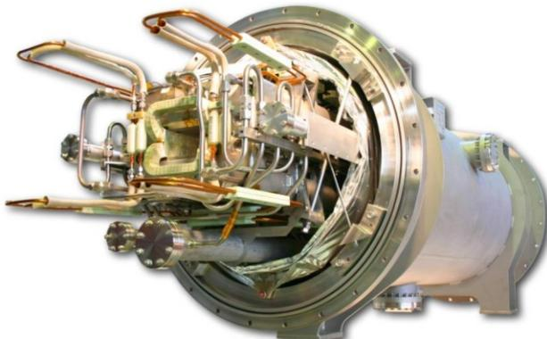
Figure 1: Photograph of the first prototype of a SIS 100 dipole magnet. The front part of the cryostat is opened to see the cold mass of the magnet. The vacuum beam pipe was inserted later.
