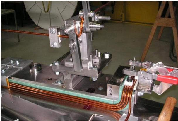
Figure 5: Photo during the winding process. The 4<sup>th</sup> turn of the inner layer is just being pre-bent to fit into the framework created by the innermost G11 pieces. Besides the coil in progress, the winding core (pre-) bending tooling and various clamping elements are visible.
