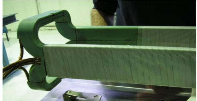
Figure 7: Photo of the double half coil during wrapping of the glass fibre tape.
