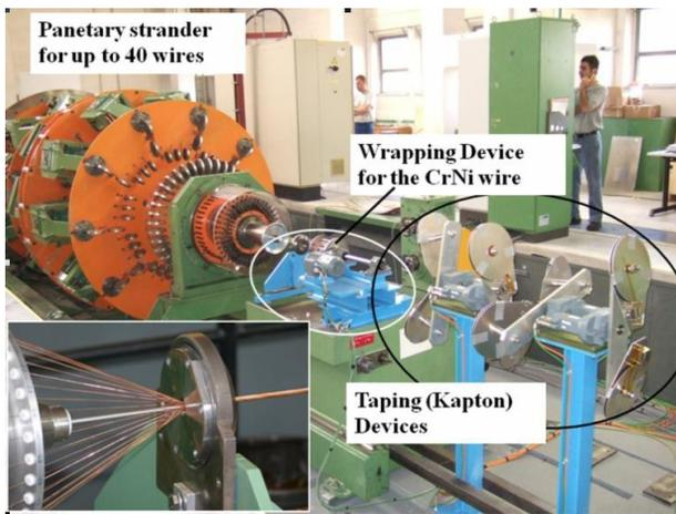
Figure 3: Cabling machine during its commissioning. From left to right: the planetary strander which can accommodate coils for up to 40 strands, the fine wire wrapping device, and the polyimide tape stations. Not shown are the caterpillar unit and the reservoir coil for the cooling tube and the re-winder for the final cable. The insert left below shows in more detail the cabling eye, where the 31 strands merge and are wound on the tube.
