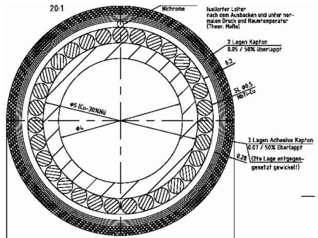
Figure 2: Schematic view of the cross section of the cable. The 31 sc strands are wound on the central cooling tube. They are kept in position and forced on the tube by a wrap of a fine wire. On the outside there are four layers (each half overlapping) of isolation tape.
