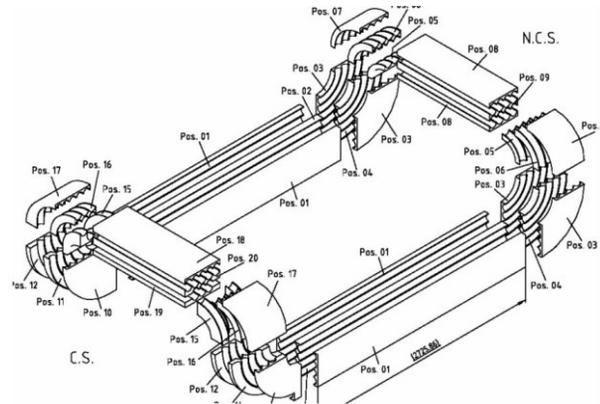
Figure 4: Exploded view of the complete set of structural elements for the upper SIS 100 dipole coil (not in scale). The coil structure (2 layers, 4 turns each) is clearly reproduced by the G11 pieces such that the cable is firmly kept all over its length.
