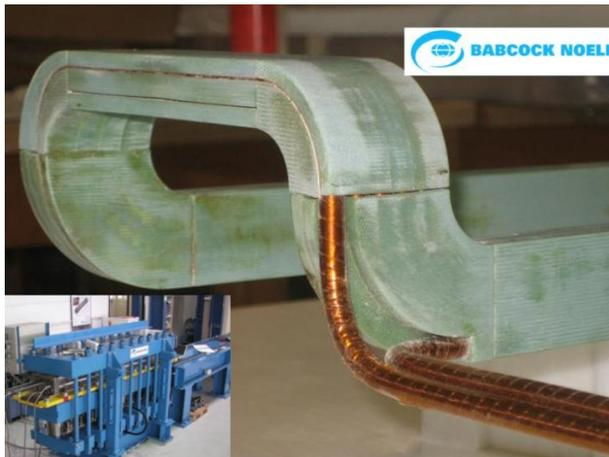
Figure 6: Photo of the head part of a readily baked coil. The insert shows the baking press which was used.
