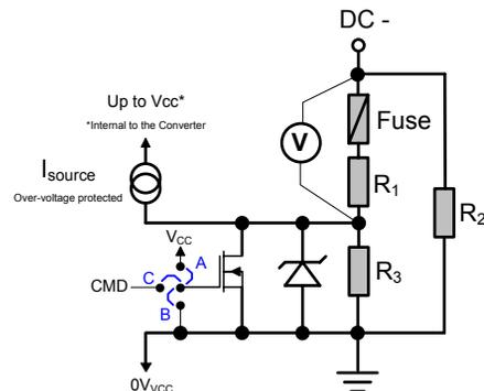
Figure 4: LHC power converter earthing circuit principle schematics.
