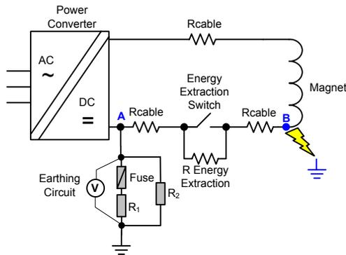
Figure 2: Passive detection.
