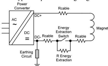
Figure 1: LHC typical superconducting magnet circuit.
