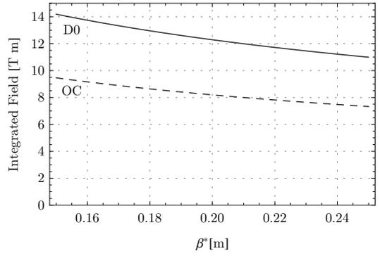
Figure 3: D0 and OC integrated magnetic field ( $IS = 5\sigma$ ,  $OS = 12\sigma$ ,  $\epsilon_n = 3.75$  mm-mrad) D0's center at 14 m and OC's center at 21 m from the IP).
