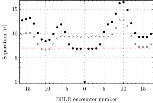
Figure 2: Comparison between an example of beams separation pattern of Table 1 scenarios C ( $\circ$ ) and D ( $\bullet$ ).
