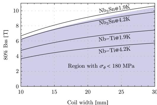
Figure 5: D0 field (80% of the short sample field) for different coil thickness, different superconductors and with respect to the mechanical limit of 180 MPa.
