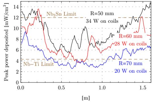
Figure 4: Power deposition result for an D0 aperture radius of 50, 60 and 70 mm (15 mm thick coils).
