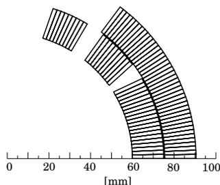
Figure 6: A possible cross section for the D0.
