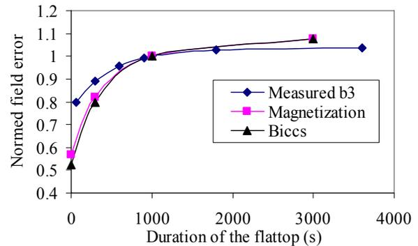
Figure 6: Comparison of calculated BICCs and magnetization decay with the measured sextupole decay.
