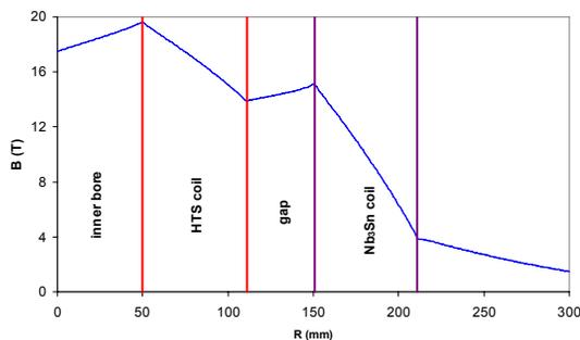
Figure 5: Maximum field in HS coil cross-section as function of the radial direction. No correction coil.
