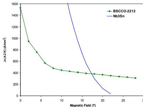
Figure 1:  $J_E$  vs.  $B$  for  $Nb_3Sn$  and Bi-2212 wires.
