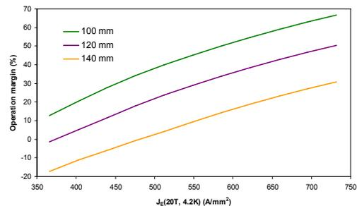
Figure 4: Operational margin as a function of superconductor (Bi-2212) engineering current density.
