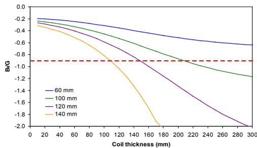
Figure 3: Helical dipole to gradient ratio vs. HS coil thickness for different coil apertures.
