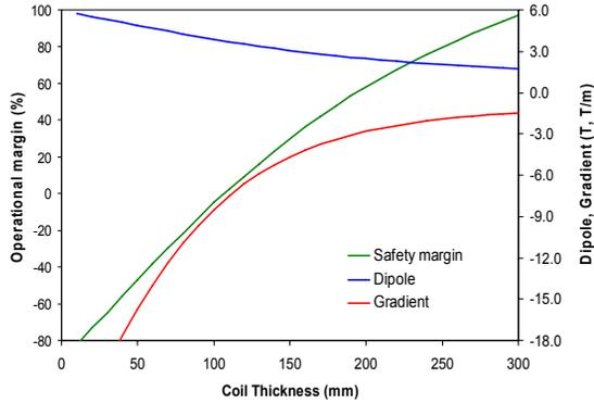
Figure 2: Operation margin, helical dipole and gradient field components vs. coil thickness.
