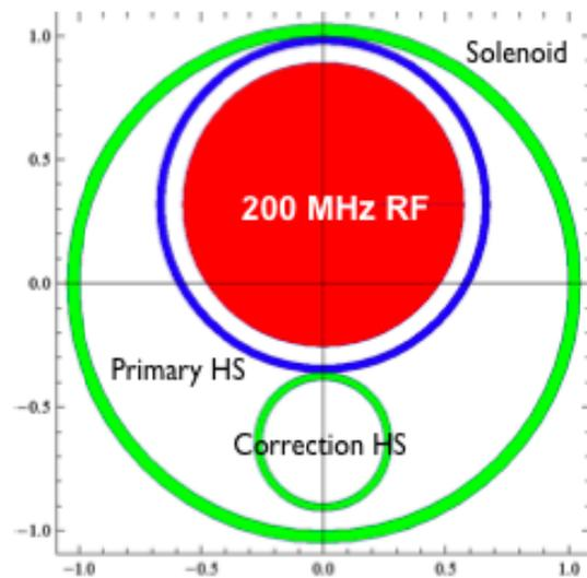
Figure 4: Schematic view of modified helical magnet with correction coils. The unit is meter. The origin is the helical magnet center.
