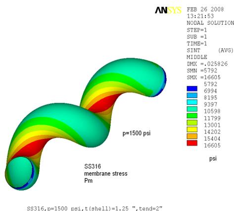
Figure 1: Mechanical analysis of high pressurized helical tube.
