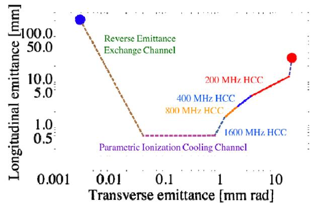
Figure 6: Transverse and longitudinal phase space evolutions in a series of HCCs.
