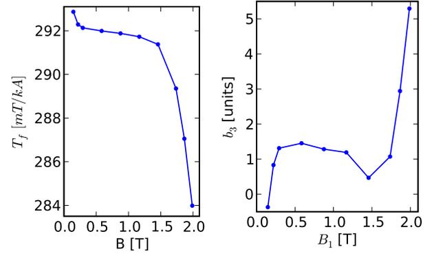
Figure 3: The transfer function of the SIS 100 dipole as well as the sextupole
