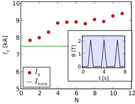
Figure 2: Quench training curve for the first prototype. The insert on the right shows the strongest cycle mode of the magnet continuously tested during one week.
