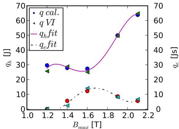
Figure 4: Dependences on  $B_{max}$  of the AC loss fit parameters  $q_h$  and  $q_e$  obtained from calorimetric and V-I measurements. The lines present the final parameter functions  $q_h(B_{max})$  and  $q_e(B_{max})$  describing the AC loss properties of the magnet according to (3).
