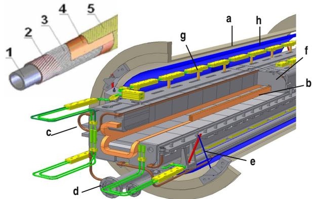
Figure 1: The structure of the Nuclotron cable (top left) and the main features of the magnet design of the first full size dipole. 1 – cooling tube, 2 – superconducting wire (multifilament NbTi/Cu), 3 - Nichrome wire, 4 – Kapton tape, 5 – adhesive Kapton tape, a – cryostat vessel, b – cable and half coil (2 · 4 windings), c – yoke cooling pipes, d – LHe lines, e – suspension rods, f – soft iron yoke, g – bus bars, h – thermal shield
