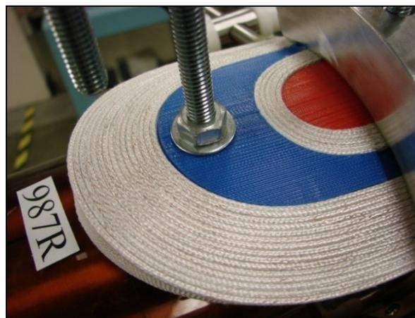
Figure 4: A practice coil using rapid-prototyping parts.
