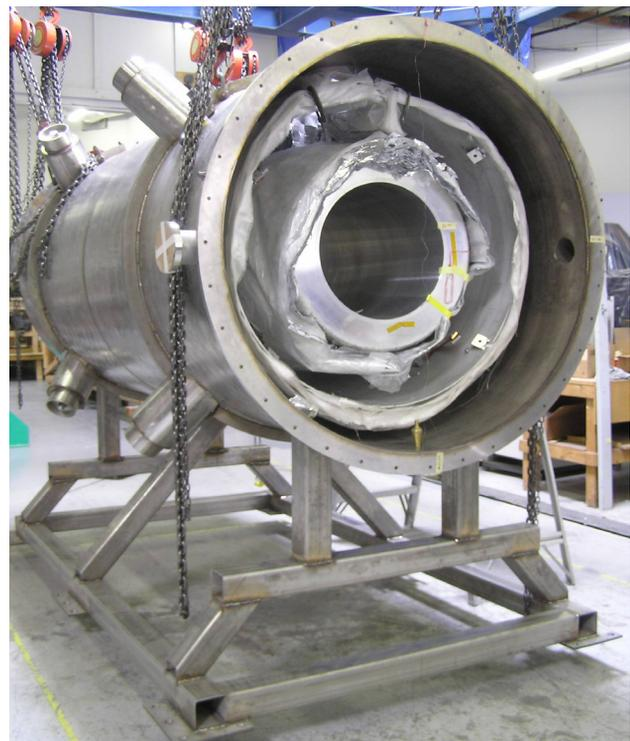
Figure 4: Magnet vacuum vessel and support stand with cold mass and radiation shield in place.
