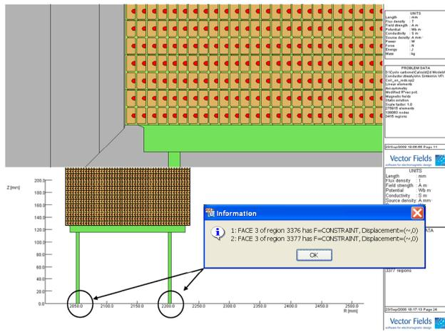
Figure 6: Full model with supports with axial boundary conditions on the support pillars.
