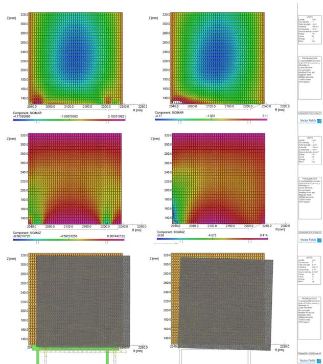
Figure 8: Comparison of radial stress, axial stress and coil displacement for a flat and tilted support.
