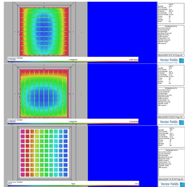
Figure 4: Radial, Axial and Hoop stresses in the macro-conductors model.
