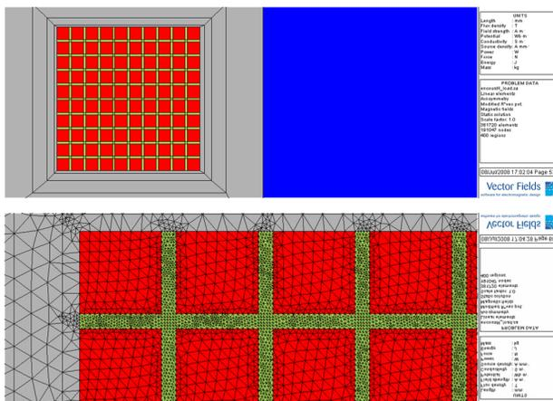
Figure 3: Subdivision in macro conductors with dense meshing in the resin.
