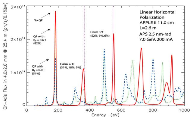
Figure 5: Flux of the APPLE-II with two quasi-periodic field-strength reductions. The reduced remanence fields  $B_r$  of 0.6 and 0.0 Tesla near the QP poles give rise to magnetic field reductions at the QP poles of 8% and 15%, respectively. Other conditions are the same as in Fig. 4.
