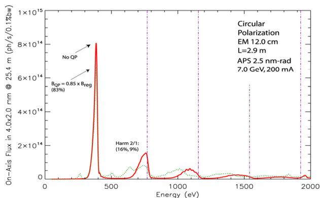
Figure 6: Flux of the EM in circular polarization mode at 400-eV first-harmonic energy. The intensity at the 5<sup>th</sup> harmonic arises primarily from the non-sinusoidal shape of the magnetic field. The other higher orders are primarily due to the size of the aperture and the beam emittance. Other conditions are the same as in Fig. 4.
