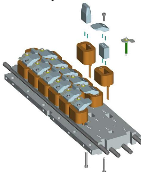
Figure 1: Split view of approximately two periods of one jaw of the EM. Both the off-centered horizontal and the centered vertical poles (blue) and the coils (brown) are shown. The poles are made of vanadium permendur. The full-length undulator is 40 periods long (4.8 m). Two end poles at each end and the quasi-periodic poles will be powered separately.
