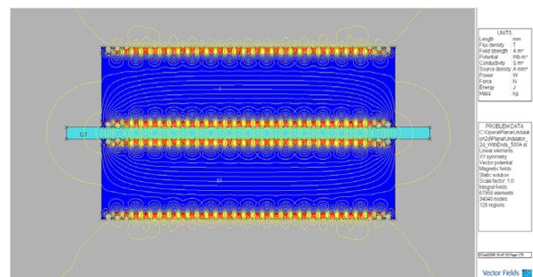
Figure 1: 2d Opera model of the undulator with coil windings shown in red and the core shown in blue. The magnetic flux lines (in yellow) are also shown.
