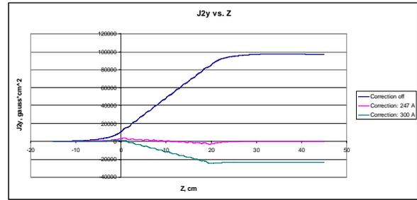
Figure 5: Effect of operating a pair of correction coils on the second field integral.
