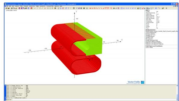
Figure 2: 3d Opera model of the undulator section with coil windings shown in red and a quarter of the core shown in green.
