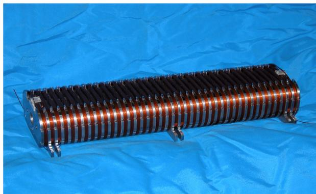
Figure 6: A 42-pole test coil wound on an assembled iron-core with iron poles.
