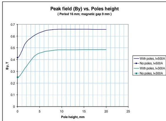
Figure 3: Dependence of peak field on the iron pole height.
