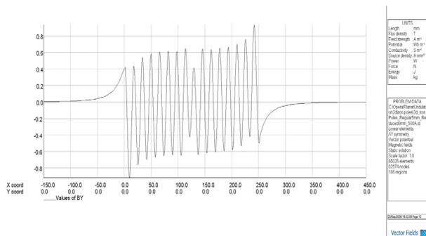
Figure 4: Simulated field profile for a short-length magnetic structure with two non-magnetic poles in the middle.
