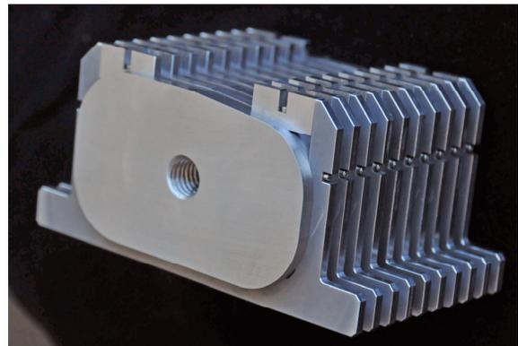
Figure 2: A 10-pole test Al core. The poles are separate pieces assembled onto the central core.
