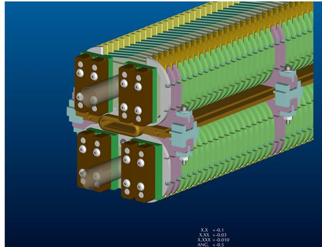
Figure 1: Magnetic structure layout of a superconducting planar undulator.
