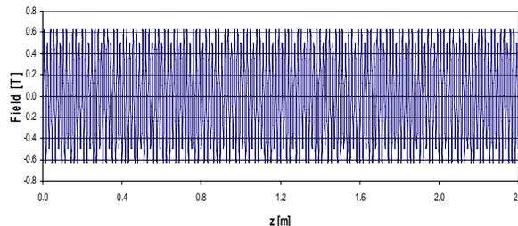
Figure 6: Magnetic field distribution along the undulator axis used in calculation of the photon flux density.
