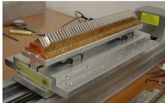
Figure 4: Magnet array on the field measurement bench.
