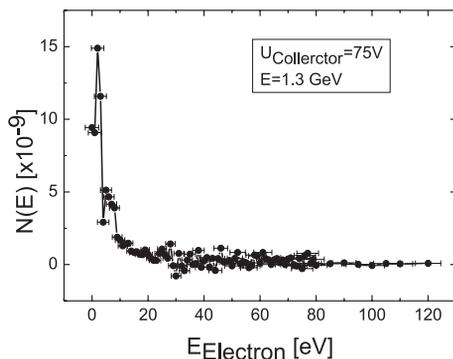
Figure 6: Electron energy spectrum at 1.3 GeV and a grid voltage of 75 V.
