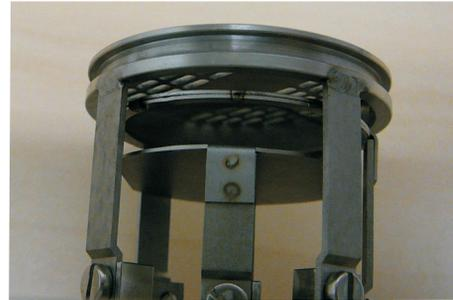
Figure 1: Picture of the in house developed retarding field analyzer.
