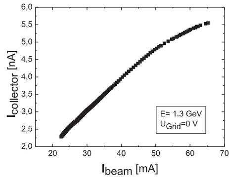
Figure 7: Collector current as a function of the electron beam current at 1.3 GeV with  $U_{collector} = 50$  V and  $U_{grid} = 0$  V.
