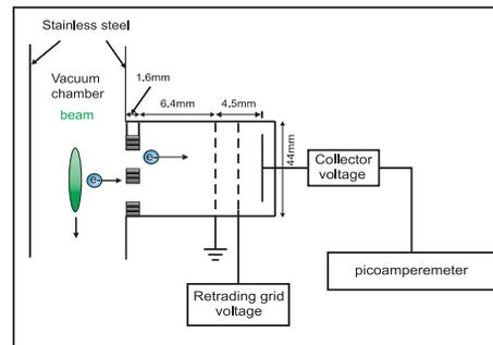
Figure 2: Sketch of the experimental set up of the RFA.
