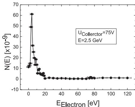
Figure 5: Electron energy spectrum at 2.5 GeV and a grid voltage of 75 V.
