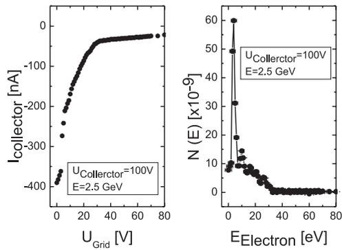
Figure 4: Measurements at the ANKA storage (beam energy 2.5 GeV, beam current approx. 110 mA, grid voltage 100 V). Left plot:  $I_{collector}$  against  $U_{grid}$ . On the right: correspondent derivative.
