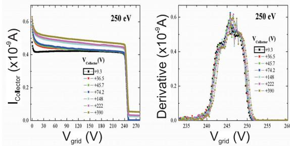
Figure 3: Results of the calibration for 250eV beam energy. Left plot: collector current over grid voltage. On right: correspondent derivative in the region when the beam energy equals the grid voltage.
