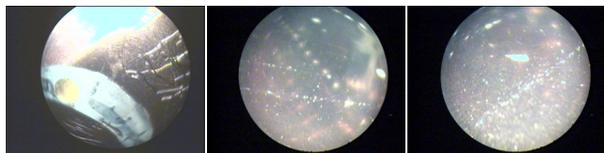
Figure 3: Pictures from inspection. Left: discoloration and missing copper around a hole. Middle: dust deposited along magnet edges. Right: Line of dust and a scratch on the surface (shiny spot)
