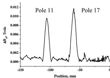
Figure 5: Correction field generated by the racetrack coils on top of the background field from the main coil operated at 186 A.
