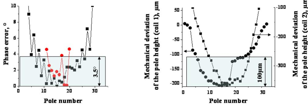
Figure 3: Left: Undulator mock-up phase errors calculated with eq. (4) (squares) and with phase function corrected for the trajectory (circles) [11] vs. number of pole at 8 mm gap. Right: measured mechanical deviations of the pole height of both coils. Two periods at both ends of the undulator are omitted.
