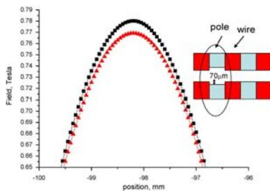
Figure 4: The difference in the peak field for one pole between the simulated ideal field (black dots) and simulated case where the pole height is decreased on both sides of the magnet by 70 μm (red) leading to the local phase error of 3.5°.
