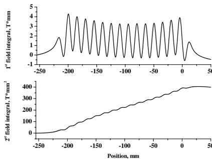
Figure 2: 1<sup>st</sup> and 2<sup>nd</sup> field integrals calculated from measured magnetic field at 186 A.
