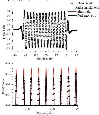
Figure 1: Above: Measured field along the central axis of the undulator with a current of 186 A.
