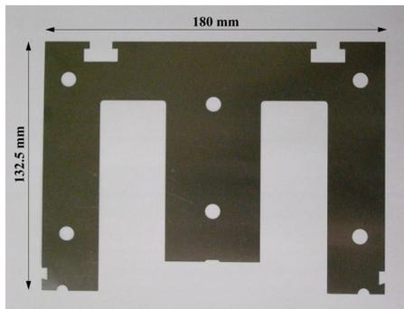
Figure 4: 0.1-mm permalloy lamination.
