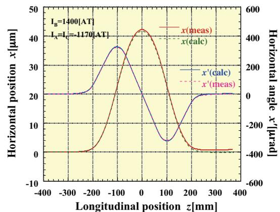
Figure 6: Beam positions and angles obtained from the field measurement and calculation at the coil currents of  $I_A=I_C=-1170$  AT and  $I_B=1400$  AT.
