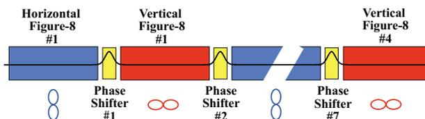
Figure 1: Schematic view of the polarization-controlled undulator.
