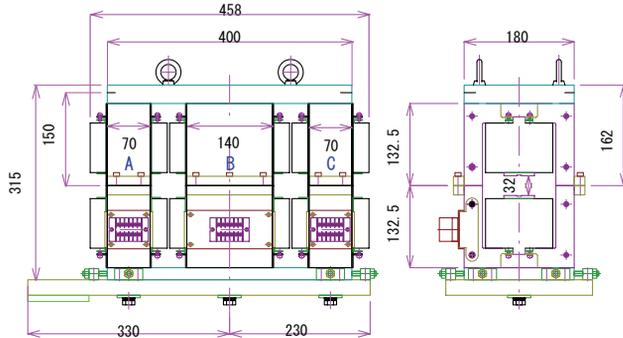
Figure 2: Plan of phase shifter prototype.
