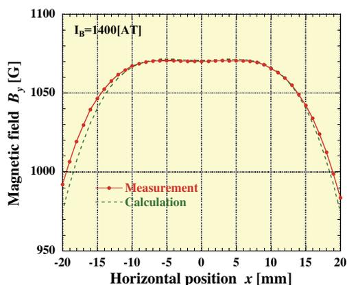
Figure 7: Measured and calculated horizontal field distributions at the prototype (Magnet B) center for the coil current of  $I_B=1400$  AT.
