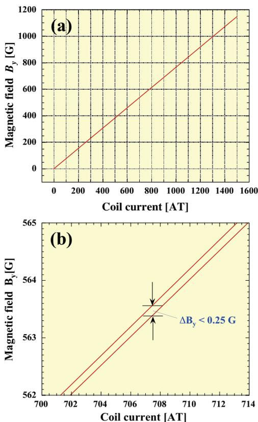
Figure 8: Excitation curve of Magnet B (a) for the coil current of 0 - 1500 AT and (b) 700 - 714 AT.
