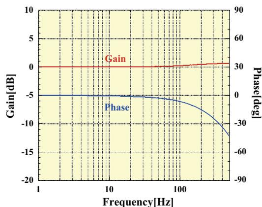
Figure 9: Measured frequency response at the center of Magnet A.
