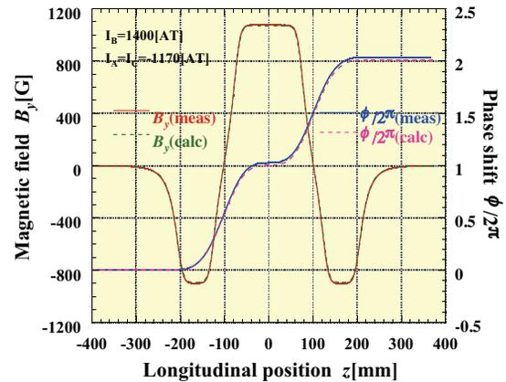
Figure 5: Measured longitudinal field distribution and its phase shift at the coil currents of  $I_A=I_C=-1170$  AT and  $I_B=1400$  AT. Calculated results of ELF/MAGIC are also shown for comparison.
