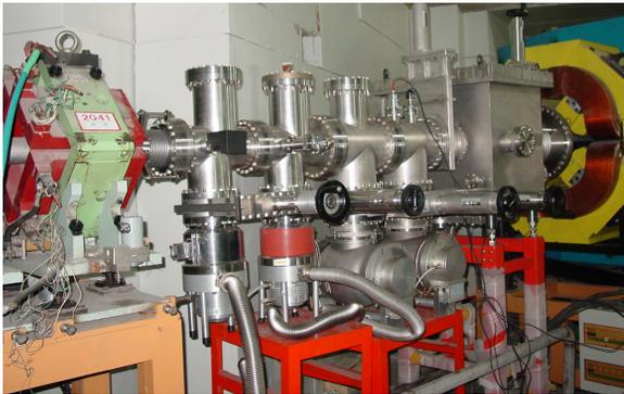
Figure 5: The differential pumping system of the Gas-filled Recoil Separator (MBP were used in 1-2 stages).
