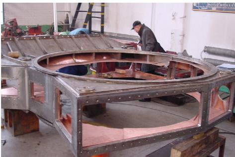
Figure 1: SFC double-deck vacuum chamber.
