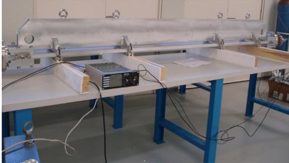
Figure 3: NEG coated Al vacuum chamber during the testing at CELLS.
