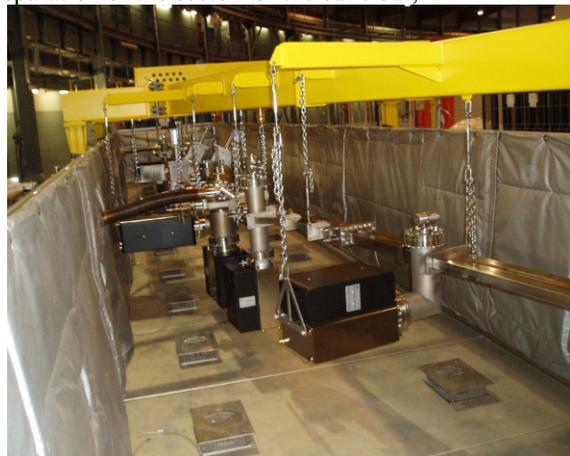
Figure 6: the sector suspended to the strong back inside the bake out oven.
