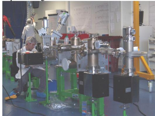
Figure 5: The assembly of the storage ring sector inside the clean room.
