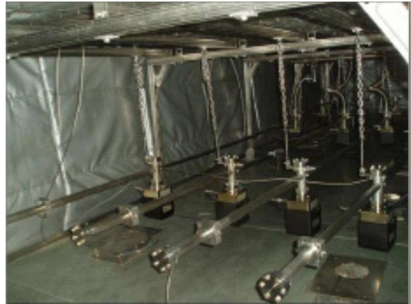
Figure 1: Four sections of the booster inside the oven prepared for bake out.
