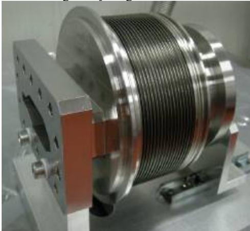
Figure 4: The bellows prototype during the movement tests.
