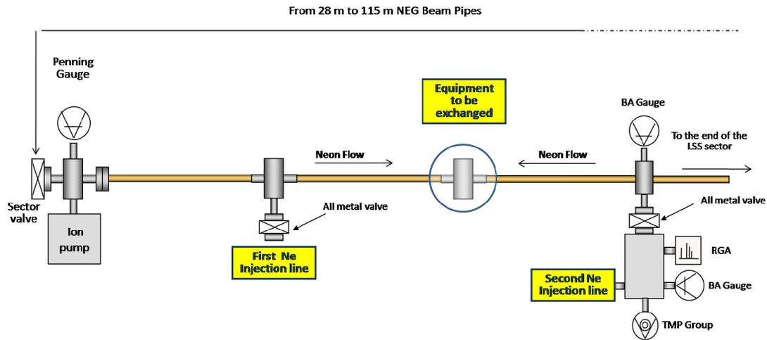
Figure 2: Schematic of a standard configuration with the two Ne injection lines.
