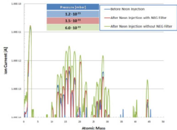
Figure 4: Spectra of the system before and after Ne injection with and without the NEG filter.
