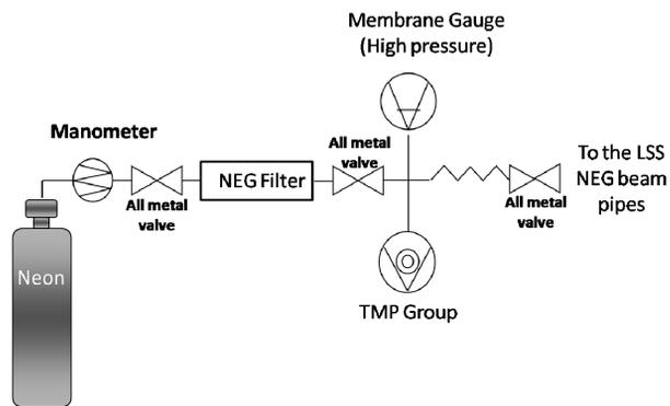
Figure 3: Schematic of the Ne injection line.
